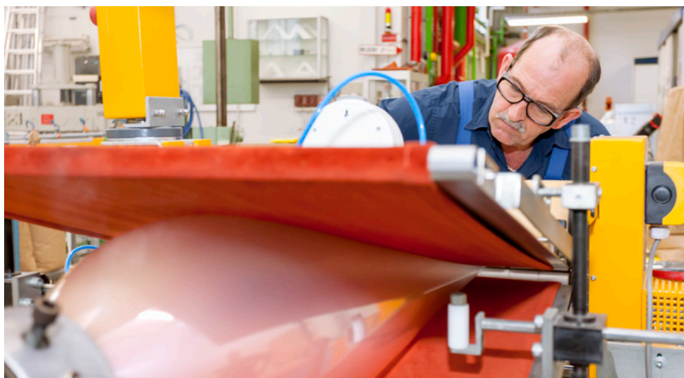
Left: At the application technology center in Burghausen all important PVC processing technologies can be replicated. In the picture a blow film extruder for the production of soft PVC films. Below: In the research laboratory in Gendorf.
