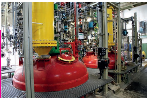
Polymerisation reactor for producing paste PVC, Burghausen
