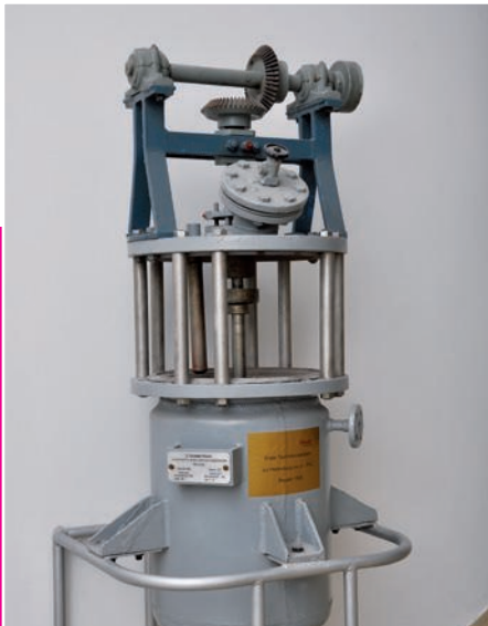
Wacker pilot plant reactor for the production of suspension PVC from 1936, Burghausen
